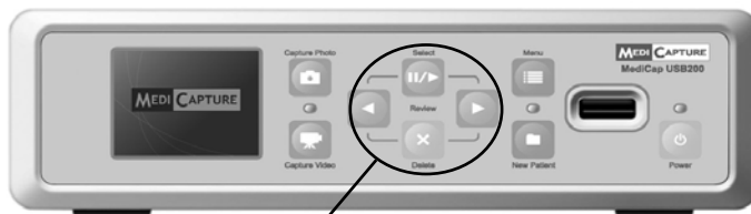
Select, Back, Next and Delete buttons are used for reviewing images and playing video.
